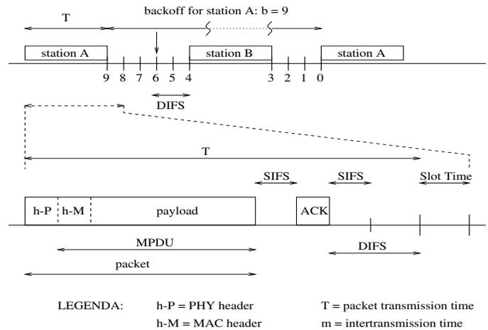
Fig. 1. Example of Basic Access Mechanism
