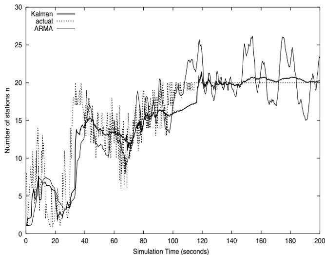
Fig. 8. Kalman filter estimation in non saturated network conditions
