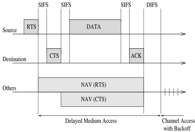
Fig. 2. RTS/CTS Access Mechanism
