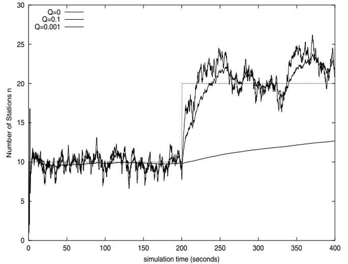
Fig. 6. Tracking ability of the filter varying the variance of the state noise
