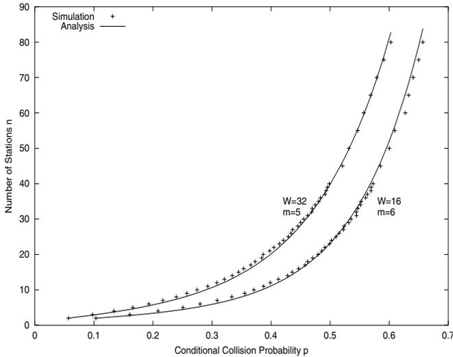
Fig. 3. Number of Stations versus Conditional Collision Probability: analysis vs simulation
