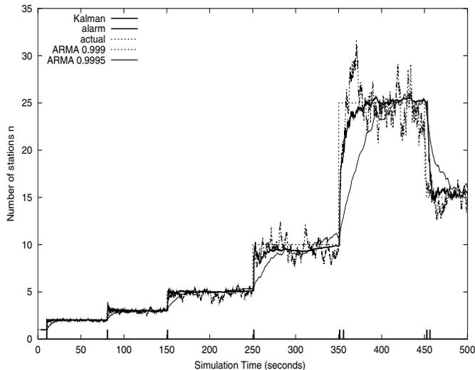
Fig. 7. Kalman filter estimation in saturated network conditions
