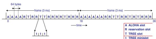
Fig. 2. Schematic representation of the frame structure.
