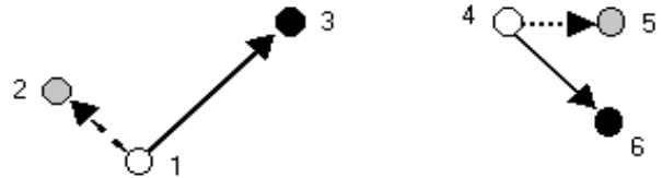
Fig. 8. Disjoint sets can be present in a multicast solution even when there are no loops.
