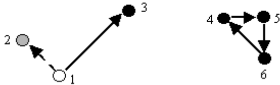
Fig. 6. Example to illustrate loops and disjoint sets. The sets \{1,2,3\} and \{4,5,6\} are disjoint. Nodes \{4,5,6\} form a loop.
