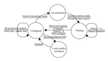
Figure 6. The finite state machine for prophet allocation
