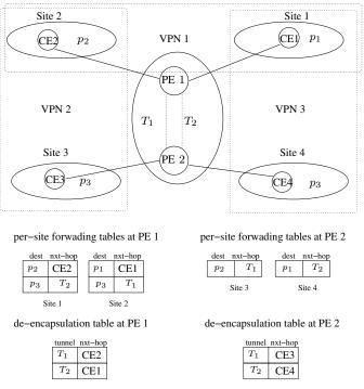
Fig. 4. Tunnels are required in the backbone.
