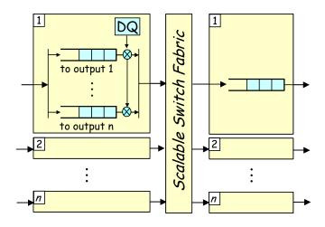
Figure 1. Simplified router diagram
