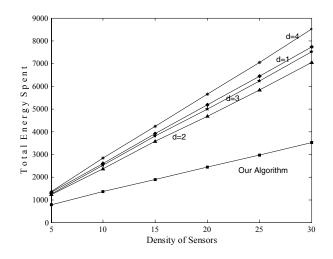
Figure 3. Comparison of Our Algorithm and the Max-Min D-Cluster Algorithms .
