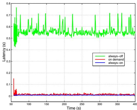
Fig. 5. End-to-end delay of one 3-hop connection, rate = 1kbps
