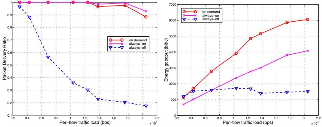
Fig. 4. Packet delivery ratio and energy goodput vs. pause time, 10 long-lived CBR connections, 50 nodes, 1500x300 static network
