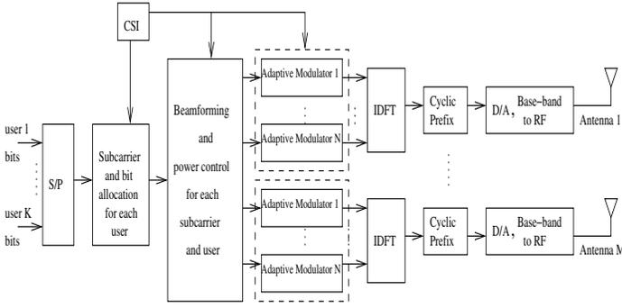
Fig. 3. Block diagram of a multi-user OFDM/SDMA transmitter.
