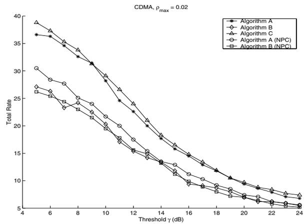
Fig. 6. Total achievable system rate vs. SIR threshold for CDMA with low code cross-correlation.
