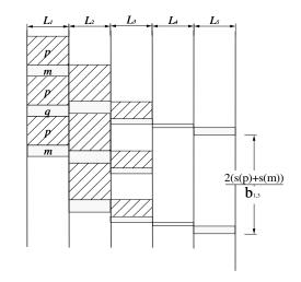
Fig. 3. Illustration of cartouche probing: A cartouche of size r = 2 is used to measure  $b_{1,3}$ . Here, the maximal spacing between marker packets m is introduced at  $L_2$  (which is the slowest link on the subpath  $L_1L_2L_3$ ) and preserved until the markers reach their target  $L_5$ .
