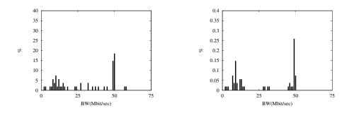
Fig. 8. Histograms of estimated  $b_{5,10}$  (left) and  $b_{5,15}$  (right) values after using a sequence of 100 cartouche trains of dimension r = 2. The setup includes 16 cross-traffic flows over each physical link, actual  $b_{5,10} = 50$  Mbps and  $b_{5,15} = 50$  Mbps.
