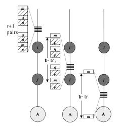
Fig. 2. A cartouche of size r consisting of back-to-back packet pairs of the form  $[pm\{pq\}^{r-1}pm]$  injected at  $L_i$  (left). Cartouche constituents are spread out over time until they arrive at  $L_j$  (middle), where only the first and last markers continue on to target A (right) with an interarrival time  $t_{\ell} - t_f = \frac{r(s(p)+s(m))}{\min_{1 \le k \le j} b_k}$ .
