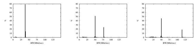
Fig. 5. Histograms of estimated  $b_{1,10}$  values after using a sequence of 100  $[pm\{pq\}^{r-1}pm]$  cartouches of dimensionality r = 1 (left) r = 2 (middle) and r = 3 (right). The setup includes 16 cross-traffic flows over each physical link, actual  $b_{1,10} = 50$ Mbps and  $b_{11,20} = 1$ Mbps.
